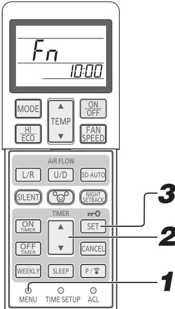
**1** Select the Fan control in heating thermo - OFF by pressing the MENU switch.
