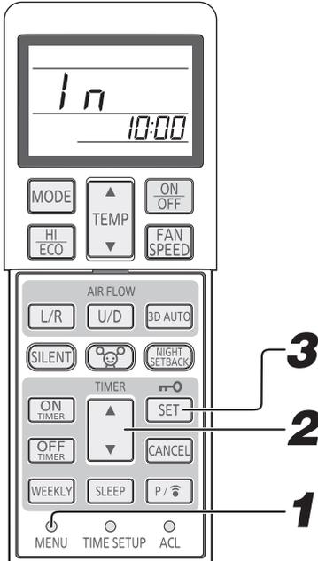
**1** Select the Wireless LAN communication setting by pressing the MENU switch.
